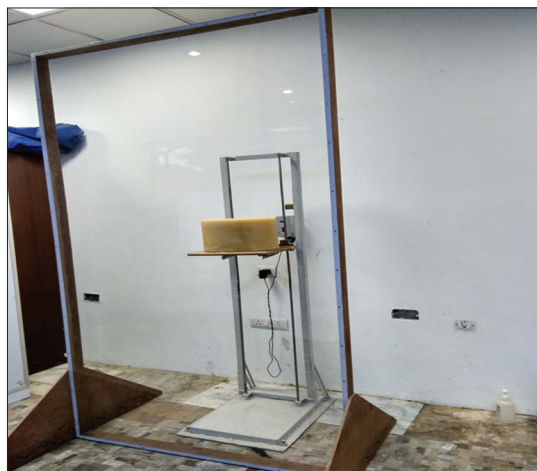
Figure 2: 6 mm PMMA and phantom stand for vertical profile movement
