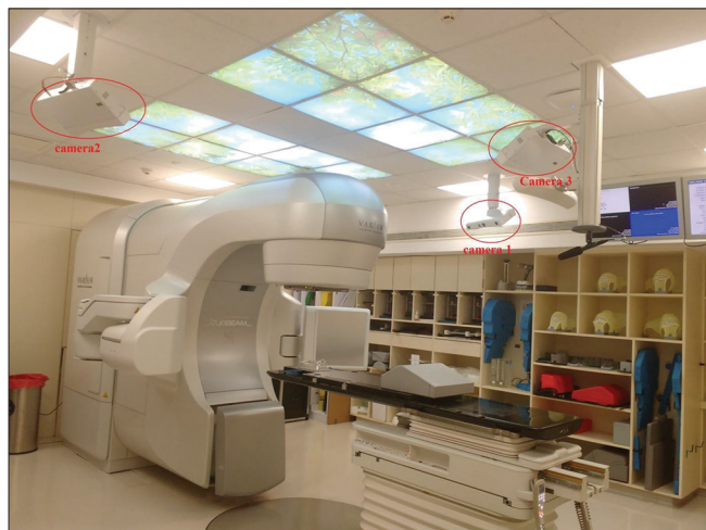
Figure 1: True Beam STX with 6DoF Perfect Pitch Couch & OSMS System
